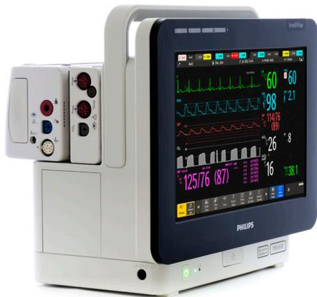
This monitor is designed to simplify clinical workflows. Since the IntelliVue MX450 can interface to other bedside devices, there's no need for a bedside device concentrator or an interface server.
